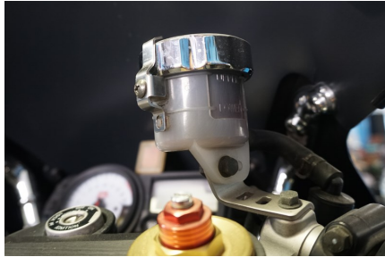
This brake fluid is old and very dark, and probably in need of being flushed. Sunlight attacks brake fluid, so it's a good idea to use a reservoir sock to cover your reservoir if it is clear.
