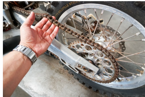
Here's a great example of a chain that was in desperate need of servicing, and probably even replacing - it was dry, rusted, dirty, and very slow to bend the links.
