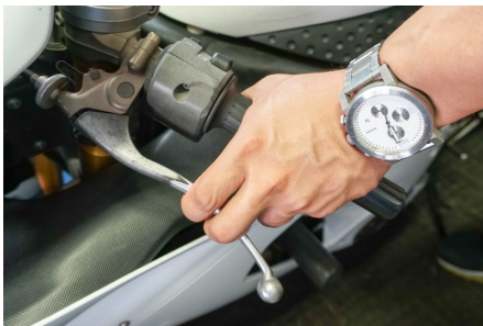
Sure enough, one of the bikes on the shop floor had this exact problem - a clutch cable that was adjusted too tight, with no slack in the lever at all. This means the clutch is always partially engaged, which will burn it out much earlier than normal.
